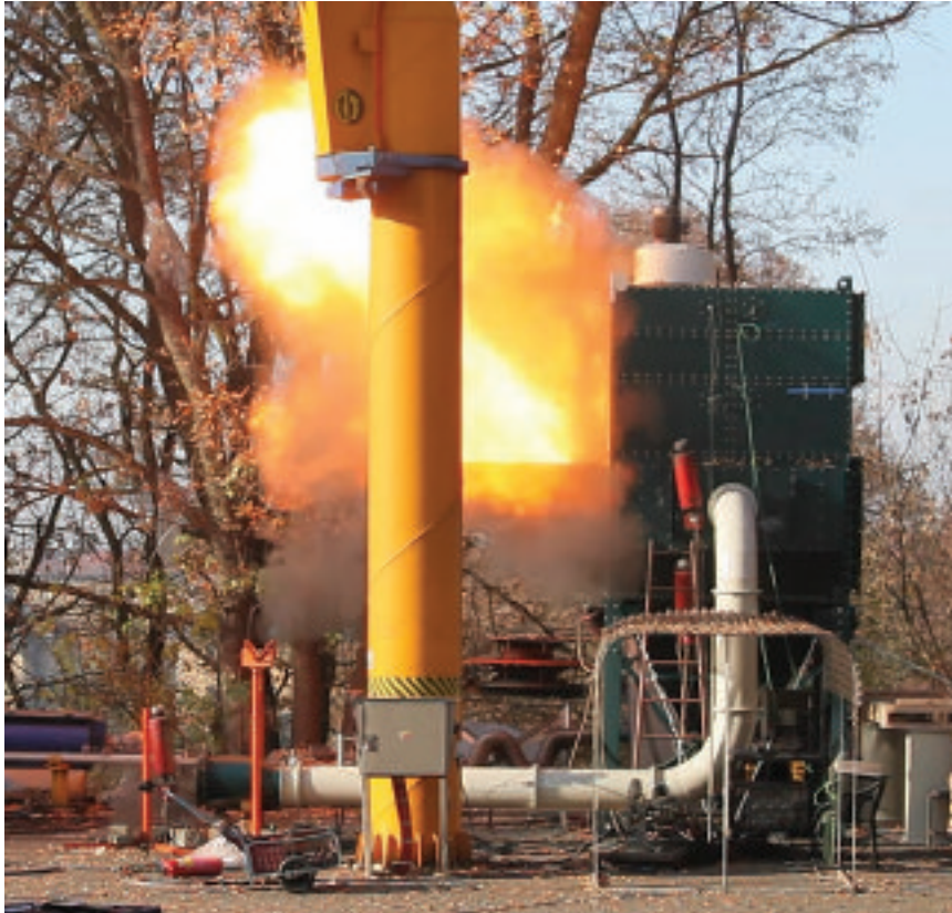
Figure 2: About 5 ms later, the dust ignites and the vent is opened. Courtesy: Camfil Farr APC
