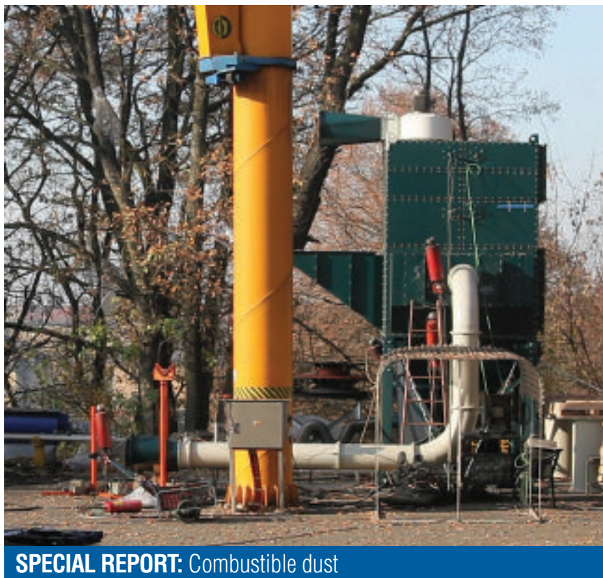
Figure 1: At the start of a dust explosion and a passive system of protection, explosive dust is injected into the dust collector to create a flammable cloud. Courtesy: Camfil Farr APC
